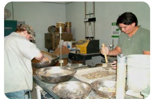
Construction Materials soil lab, preparation of proctor soil samples for compaction testing
