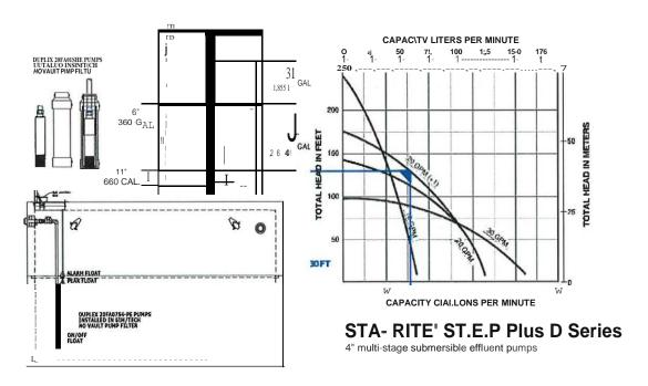
Measurements are form the tank bottom and then between floats. The available storage below the float is shown:
