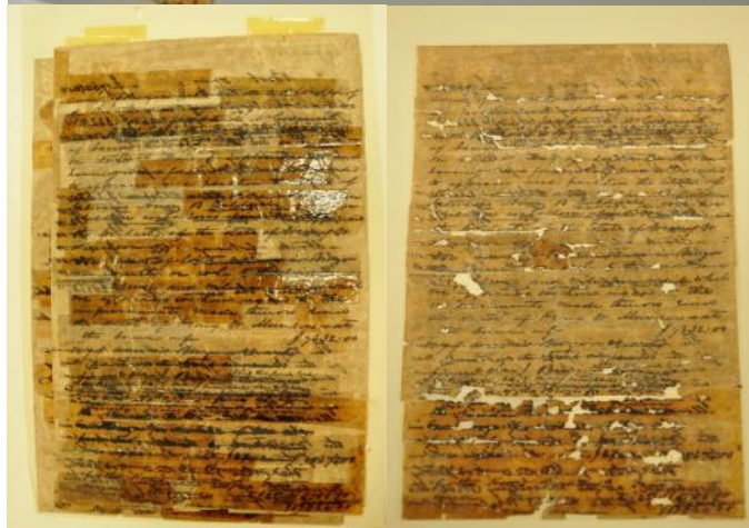
An 1848 Probate Record before (L) and after (R) treatment and mending with Japanese tissue. Above, a Kofile conservator pieces the document together after the tape was reduced.
