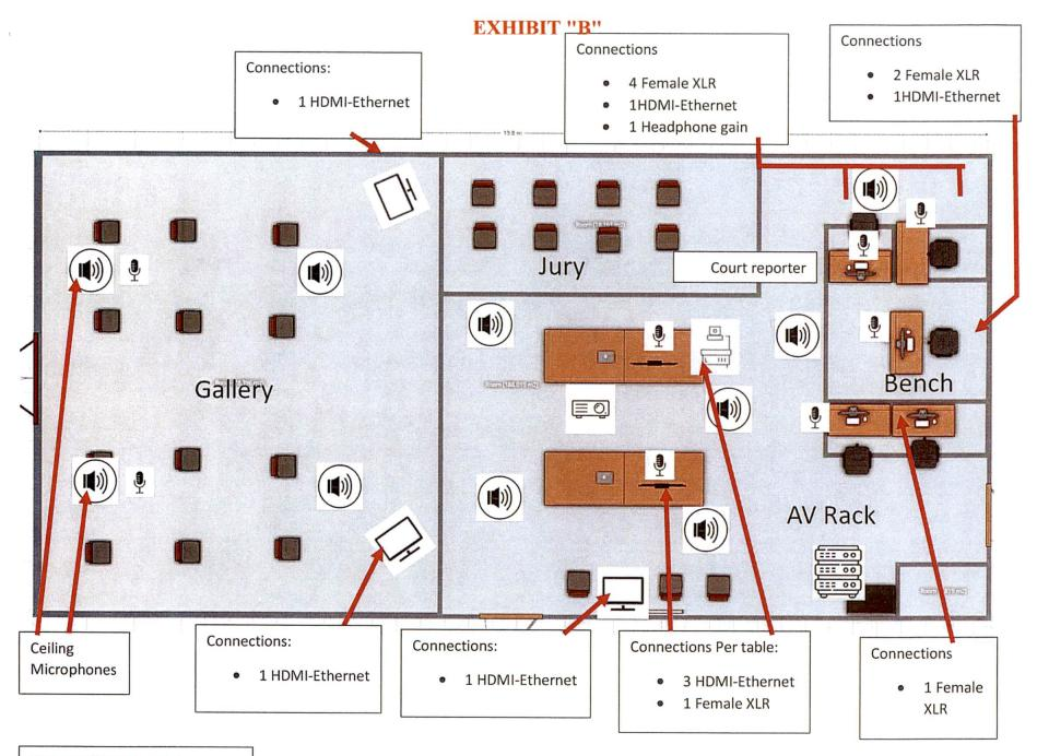
**Current System**: This layout is the current system diagram for devices.
